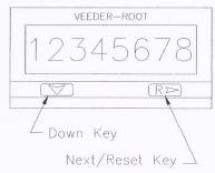
Programming parameters can be accessed by pressing the Down Key. To edit a parameter use the Down key to scroll until the desired parameter appears on the screen. Pressing the Next key will cause the leftmost digit of that value to begin to flash. Use the Next and Down keys in combination to choose individual digits and change their value.
